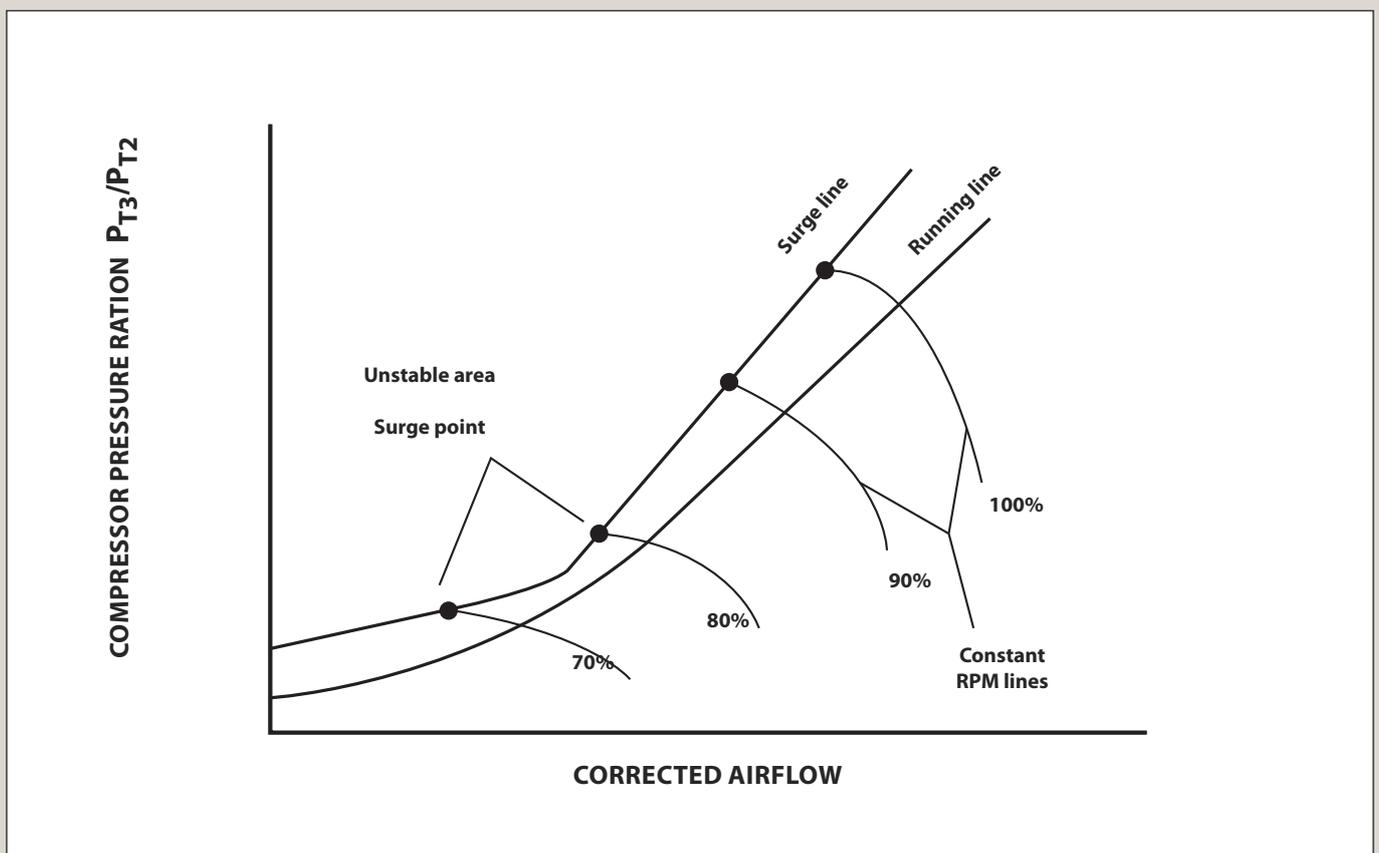
Clearly, each compression system has a degree of tolerance and the consequences of changes to conditions will depend on the way the compressor control logic works. However, changes to gas conditions can cause changes to compressor system performance. For example, for the same feed condition, compression ratio and compressor speed:
