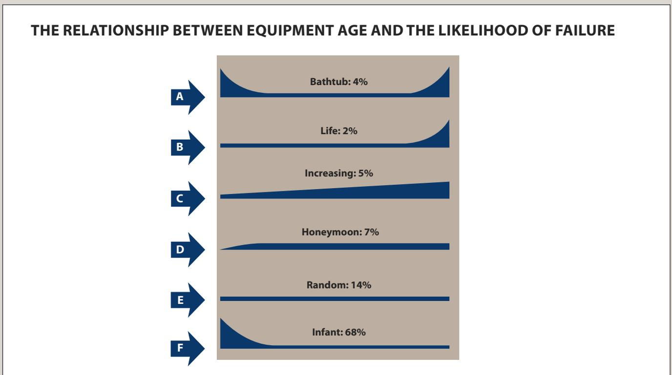
This caused a dramatic rethink in the way the aircraft industry approached maintenance and one of the outcomes was the avoidance of interference by placing a much greater emphasis on predictive/condition-based techniques. Such techniques include performance monitoring and condition monitoring such as vibration, temperature and oil monitoring, the objectives of which are to determine if there are ‘potential failures’ or warnings that something is failing.
